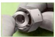
When using an Original-style Gasket, place it into the female nut whenever possible. No special positioning is needed because the gasket is self-aligning.
