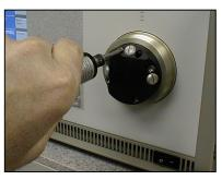
On the extended low range (LX) model, the optical assembly is attached with four hex retaining screws. Carefully remove them with the torque tool provided with your instrument. The four screws are captive within the optical head assembly and will not fall out. For all other models, only the cover screw or retaining bar holds the optical assembly.
