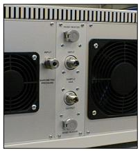
The input and output connectors are clearly labeled on the Sample Gas section of the back panel. Depending on the specific model and ordered options, the stainless steel gas input and output connections may be 6 mm Swagelok, 1/4 inch Swagelok, or ¼ inch Cajon VCR.
