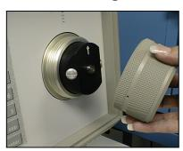
The heart of the 373 Dew Point Mirror instrument is the measuring head assembly. It is designed to be highly sensitive and accurate, yet rugged and easily accessible for periodic mirror cleaning. Although not required prior to initial operation, you may wish to familiarize yourself with the location and accessibility of the mirror and the other optical components within this assembly.
