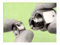
Removing VCR components in an assembled system requires no axial clearance. To disassemble a VCR connection, hold the male nut or body hex stationary with a backup wrench and loosen the female nut. After removing the components, be sure to protect the sealing beads with protective caps or Gasket Retainer Assemblies.
