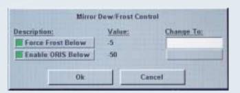
The 373 can automatically force all sub-zero condensation to a known state of frost, and thus eliminate the problem. Frost is ensured by rapidly cooling the mirror to below -40°C forcing the condensate to solidify, then quickly returning it to the previously predicted frost point temperature. It is then allowed to stabilize while ensuring the mirror temperature remains below 0°C. Once forced to
