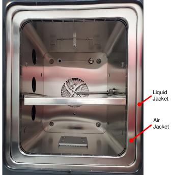
silicone profile seal for perfect tightness. An integrated chamber fan provides internal air circulation which ensures uniformity and stability throughout the working volume.
