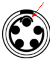
Red Dot aligns with Pin 1
