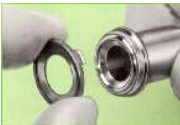
When using a Gasket Retainer Assembly, press the assembly onto the gland as shown. The retainer assembly will locate the gasket over the bead and hold it in place. Be careful not to scratch or nick the bead. Damage to the bead may cause leakage.
