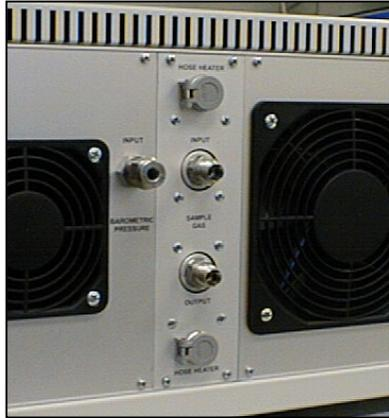
The input and output connectors are clearly labeled on the Sample Gas section of the back panel. Depending on the specific model and ordered options, the stainless steel gas input and output connections may be 6 mm Swagelok, ¼ inch Swagelok, or ¼ inch Cajon VCR.
