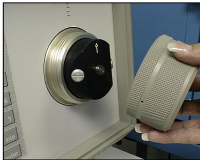
The measuring head is located on the right side of the 373 front panel. To gain access to the mirror and opto-electronic components, you must first remove the cover screw or the retaining bar. The method you use depends on the type of cover provided with your system.
