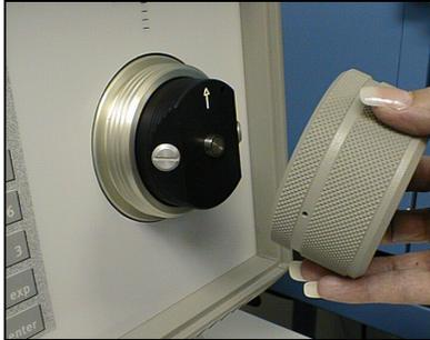
The heart of the 373 Dew Point Mirror instrument is the measuring head assembly. It is designed to be highly sensitive and accurate, yet rugged and easily accessible for periodic mirror cleaning. Although not required prior to initial operation, you may wish to familiarize yourself with the location and accessibility of the mirror and the other optical components within this assembly.
