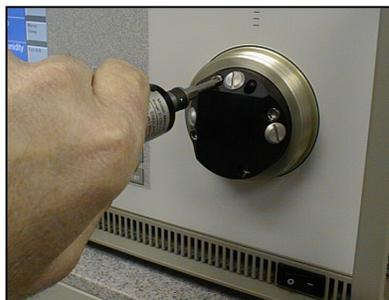
On the extended low range (LX) model, the optical assembly is attached with four hex retaining screws. Carefully remove them with the torque tool provided with your instrument. The four screws are captive within the optical head assembly and will not fall out. For all other models, only the cover screw or retaining bar holds the optical assembly.
