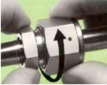
To assemble the connection, hold the male nut or body hex stationary.
