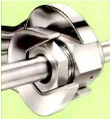
Hold the male nut or body hex stationary with a backup wrench. Tighten the female nut 1/8 turn past finger-tight for 316 stainless steel and nickel gaskets or 1/4 turn past finger-tight for copper and aluminum gaskets.
