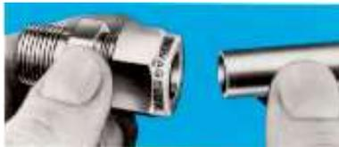
Simply insert the tubing into the SWAGelok® Tube Fitting. **Make sure that the tubing rests firmly on the shoulder of the fitting and that the nut is finger-tight.**
