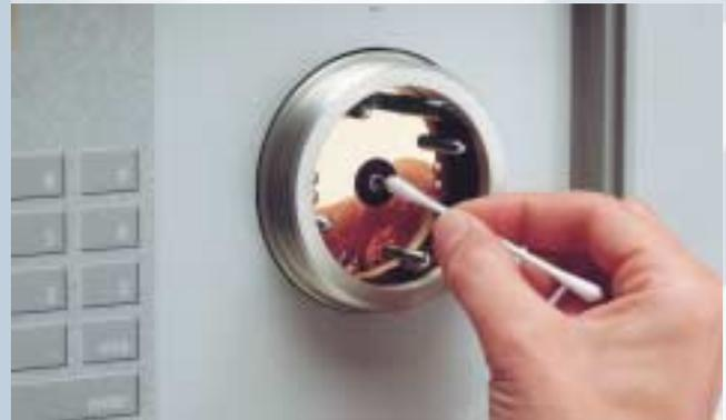
The mirror is mounted right on the front panel making it easily accessible for cleaning. Simply twist and remove the cover to gain complete access to the removable optical assembly and the flush mounted mirror surface.
