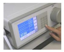
Press and hold the *Enter* key on the numeric keypad for 3 to 4 seconds. If you've done it correctly, you'll hear two short beeps and a key in the upper right corner will turn yellow. If not, release the *Enter* key and try again.
