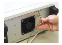
Disconect the quick coupling from the  $SAMPLE\ GAS$  inlet or connect the instrument to a  $SF_6$  reclaimer.
