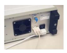
If you intend to transfer the measured data via the serial interface to a computer, the provided serial cable must be connected to the RS 232 port on the 973 and to the serial interface of the computer.
