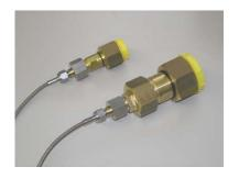
Make sure that a DILO coupling DN8 or DN20 is properly installed on the sampling tube, but do not connect the DILO coupling to anything else at this time. Since the DILO couplings are self-sealing, the sampling tube is sealed.
