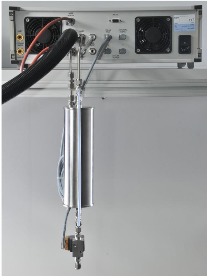
When the sample gas with a high dew point passes through the steam trap, excess water vapor condenses and is collected. The remaining gas can then pass through the 573 flow meter and sample pump without flooding. Users can also implement their own steam trap within existing installations or sampling systems. See chapter 4.4 'Back Panel' on page 23 for electrical connection of the steam trap.
