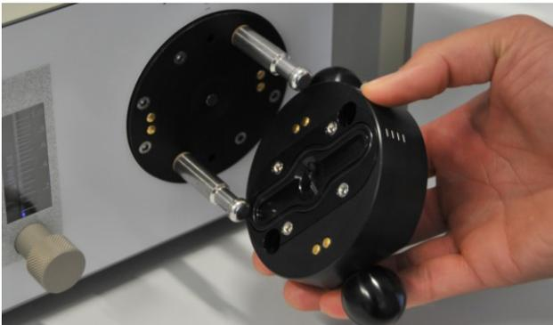
This part contains the opto-electronic components. An oval-shaped O-ring seals the measuring head. Gold contacts are located on the surface. Please avoid touching the surface of the optical unit with your fingers to avoid contamination of the contacts, the O-ring, the optical zone and the gas channel.
