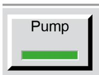
As the 573's measuring head is internal, to obtain a representative sample of the room air, flow through the measuring head is required. Press the **Pump** button to generate gas flow. Pump power can be varied, see chapter 5.4.7 'Pump' on page 40.
