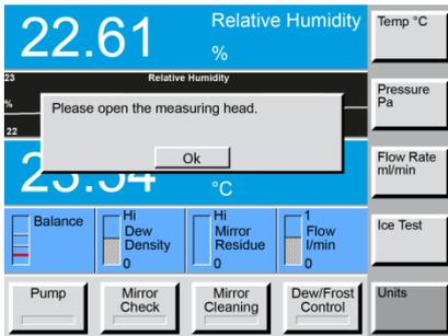
Press the **Ice Test** menu key. A window requests you to open the measuring head.
