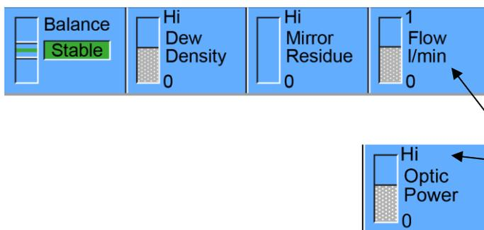
Near the bottom of the display is the Status Line. The Status Line displays **Balance**, **Density**, **Mirror Residue**, and **Flow or Optic Power**.
