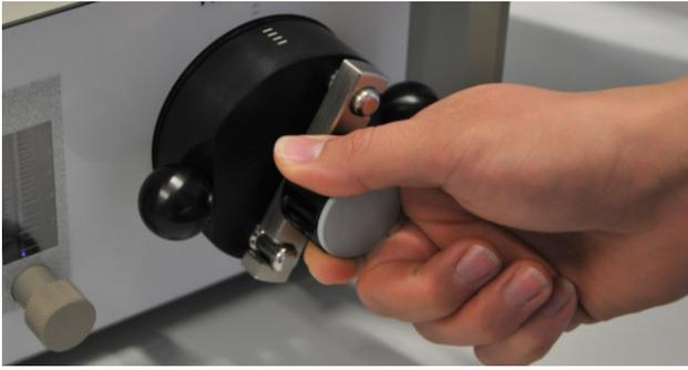
The measuring head of the dew point 373 is located on the right side of the front panel. To access the mirror or the other optical component to be removed, first, remove the measuring head clamp.
