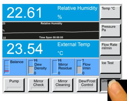
Press the menu selection key on the lower right to select the **Diagnostics Functions** menu. Then press the **Ice Test** button.
