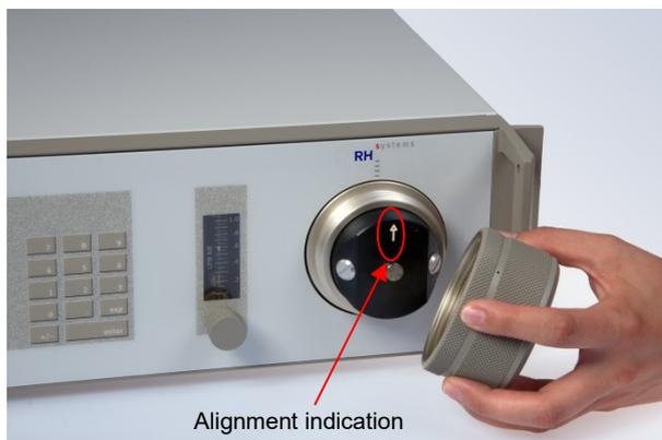
1. Install the optical assembly, taking note of guide pin (s) and alignment indication
