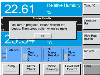
During Ice Test, the mirror rapidly cools to approximately -30 °C. Because the measuring head is open, humidity from the ambient air starts to condense on the mirror. This forms a frost layer on the mirror which can be increased if necessary by breathing on it. After reaching the low temperature and forming ice on its surface, the mirror begins to heat. As the temperature approaches 0 °C, the instrument will beep increasingly rapidly as the mirror gets closer to the ice-melt temperature.
