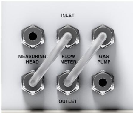
Check that the back panel sample connections are in place as shown. This is the standard set up of the 573 back panel connections.
