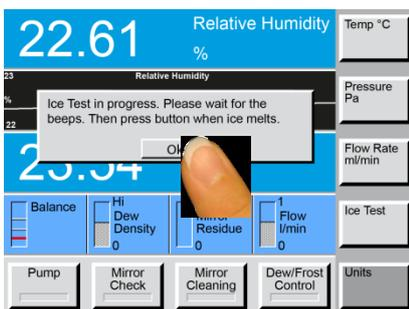
When you see the phase transition on the mirror, press the **Ok** button. The mirror temperature is measured at that moment and a dialog box appears with the test results.
