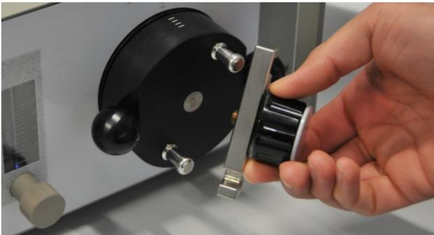
Once the clamp is removed, the black optical unit can be easily removed as shown.
