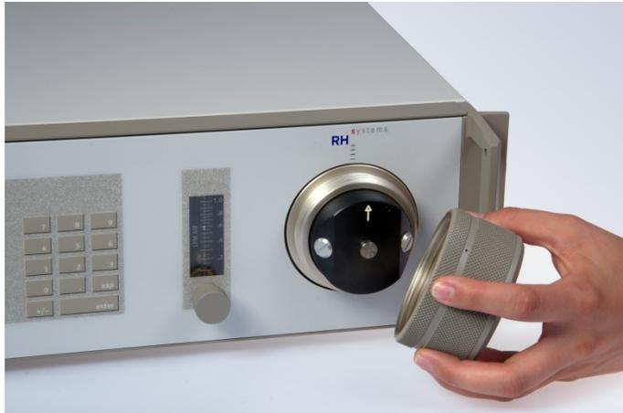
The measuring head is located on the right side of the 573 front panel. To gain access to the mirror and opto-electronic components, you must first remove the cover screw by twisting it counter clockwise. It requires approximately three full turns to completely unscrew, allowing you to remove it.
