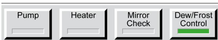
The bottom line of the display contains a row of fixed function keys. These keys are used to start and stop the **Pump**, prepare for **Mirror Cleaning** (573S only), toggle the **Heater** on/off (573H and HX only), initiate a **Mirror Check**, and switch **Dew/Frost Control** on/off.
