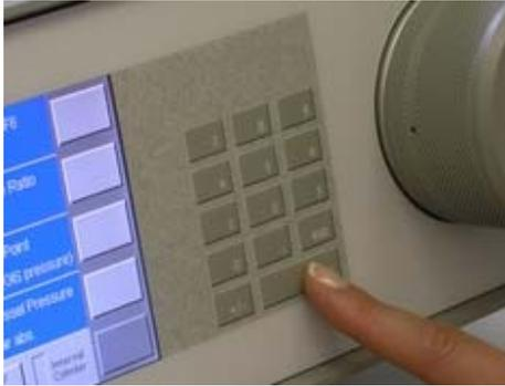
The keypad is used for entering data into the 973. For normal operation it is rarely used.
