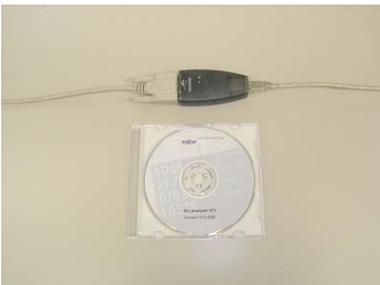
If your computer is equipped with a USB interface, you must use the provided RS 232/USB converter. You will find the drivers on the CD. The installation will be explained in the following chapter.
