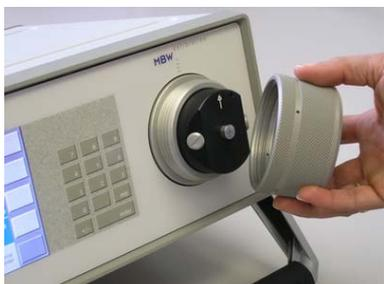
The measuring head is located on the right side of the 973 front panel. To gain access to the mirror and opto-electronic components, you must first remove the cover screw.
