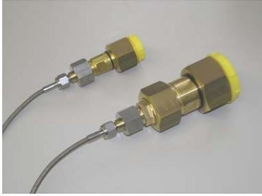
Make sure that a DILLO coupling DN8 or DN20 is properly installed on the sampling tube, but do not connect the DILLO coupling to anything else at this time. Since the DILLO couplings are self-sealing, the sampling tube is sealed.
