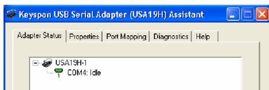
In the **Adapter Status tab**, the assistant will show you which COM Port the USB Adapter will use. You will need this COM Port number later since it will need to be entered into the ABB Excel Protocol in the cell **Read Data From COM**.
