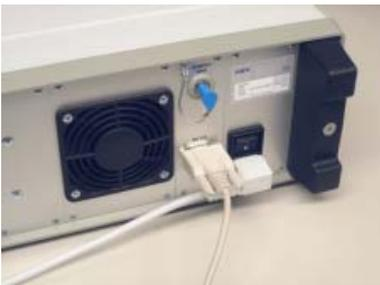
If you intend to transfer the measured data via the serial interface to a computer, the provided serial cable must be connected to the RS 232 port on the 973 and to the serial interface of the computer.
