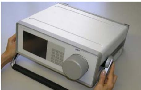
To adjust the position of the carrying handles press the buttons on both sides to unlock the handle. Release the buttons when the desired position is found.
