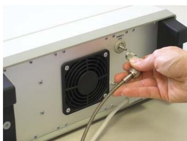
Disconnect the quick coupling from the **SAMPLE GAS** inlet or connect the instrument to a SF<sub>6</sub> reclaimer.
