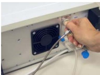
The quick coupling on the instrument side of the sampling tube must be connected to the **SAMPLE GAS** inlet.
