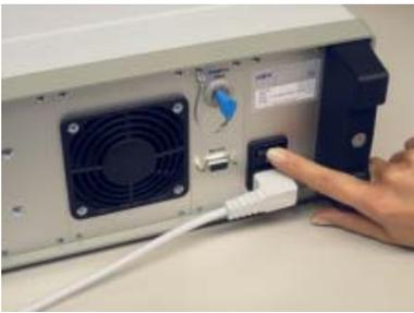
The power socket and the 973 main power switch are on the back panel of the instrument. Use the provided power cable to connect the instrument to the mains power.
