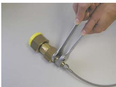
For a possible change of the DILO coupling use the supplied spanner 17/22 mm and 22/24 mm.
