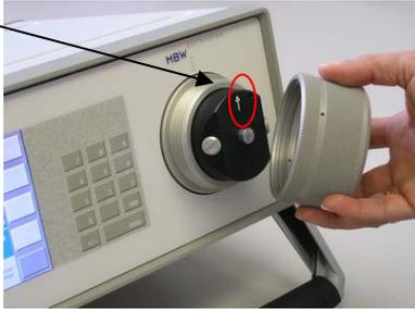
Reassemble the mirror components in the reverse order of disassembly.
