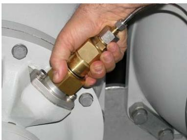
If the sampling tube was properly evacuated before the first measurement, it is now ready to connect to the gas compartment. When moving the connection from compartment to compartment, there is no need to re-evacuate.
