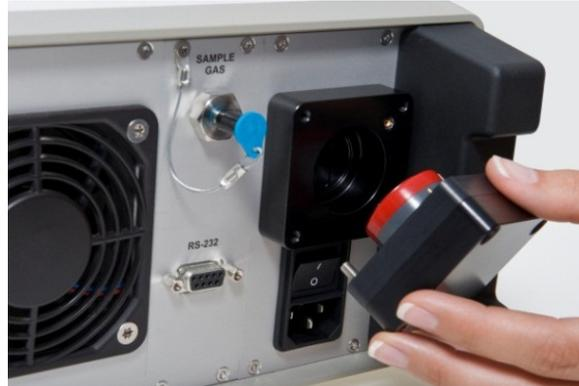
As an option, the 973-SF<sub>6</sub> is now available with integrated, industry standard chemical-based SO<sub>2</sub> measurement – another indicator of potential problems within gas-insulated equipment. The measurement cell is conveniently located on the rear panel for easy user replacement when needed (about every two years). Low cost, pre-calibrated, interchangeable modules make this swap-out a simple, two minute field operation.
