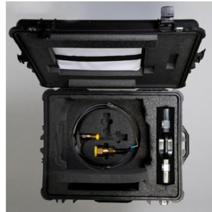
transportation. Sample lines and the most common DN8 and DN20 fittings are included. Alternative fittings are available to suit almost any SF<sub>6</sub> installation.
